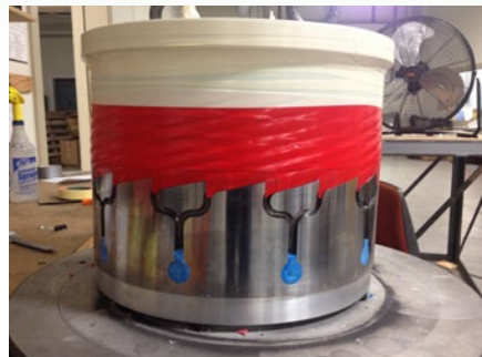
170-10s Red and HVMC - High Velocity Masking Compound (blue)
